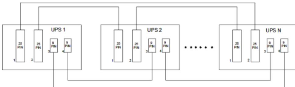
Figure 3-11: Diagram of Parallel Signal cable Connection
