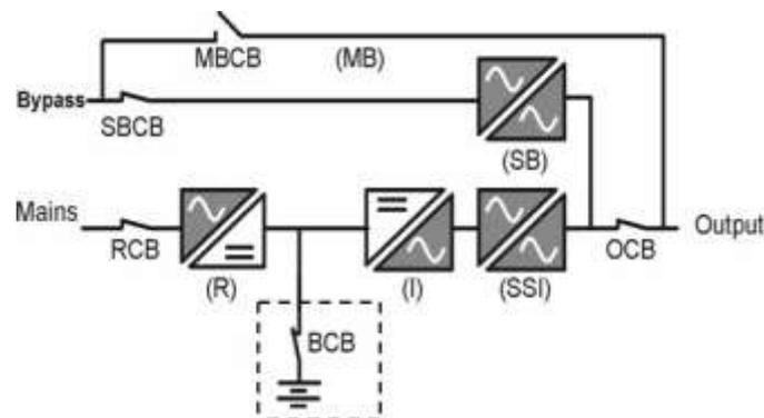
Figure 2-1: Stand-alone System Functional Block Diagram
