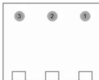
Figure 3-18: Pin Arrangement of Dry Contact OUT 1—8 Interface
