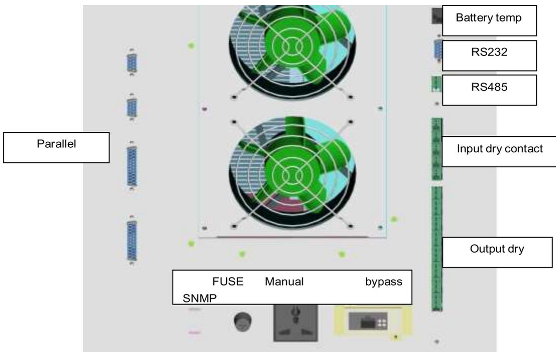
Figure 2-13: 10 ~ 40KVA communication interface diagram
