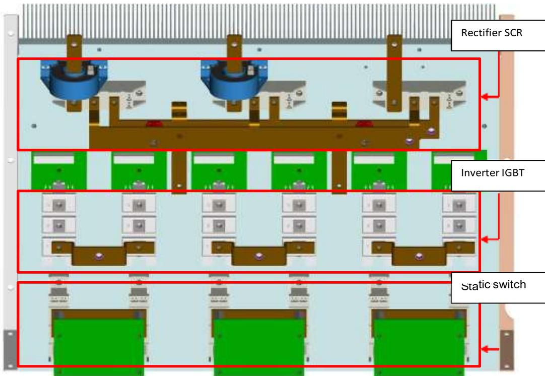
Figure 2-15: 60KVA UPS rectifier, Inverter, and STS Module
