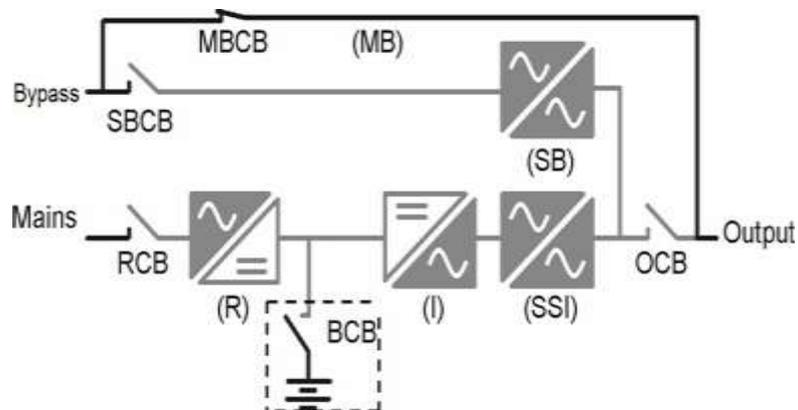
Figure 2-5: Maintenance Bypass Mode
