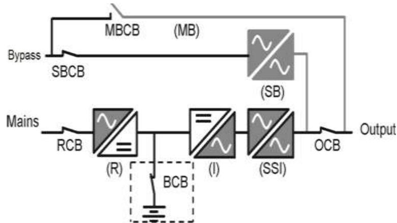
Figure 2-2: Main Power Supply Mode
