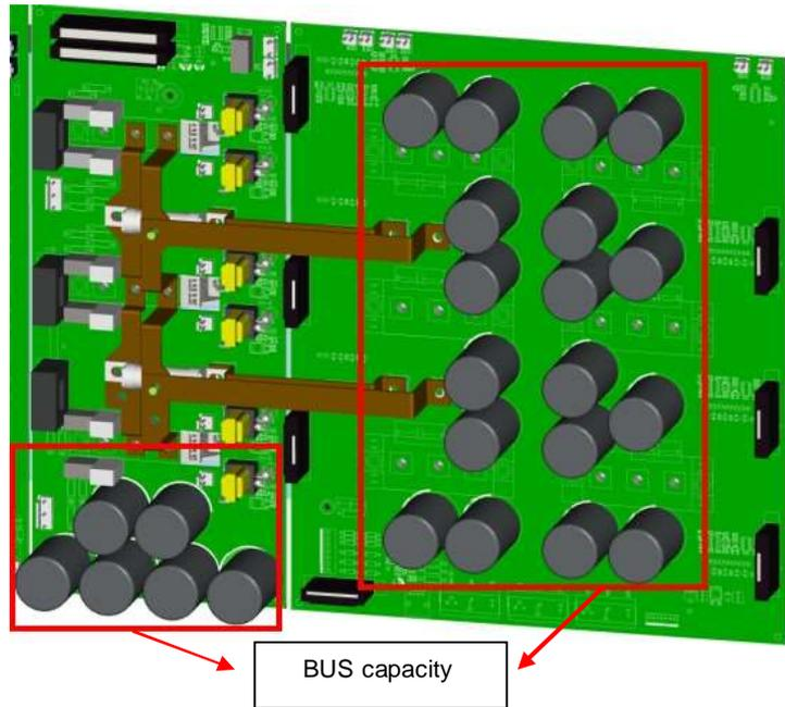
Figure 2-10: 10 ~ 40KVA BUS capacitance
