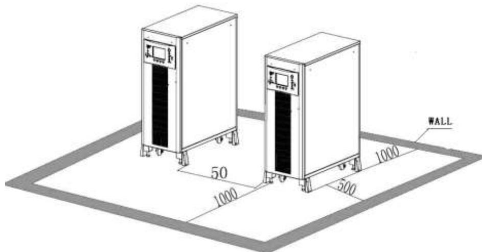
Figure 3-3: 10 ~ 40 KVA installation diagram (Unit: mm)
