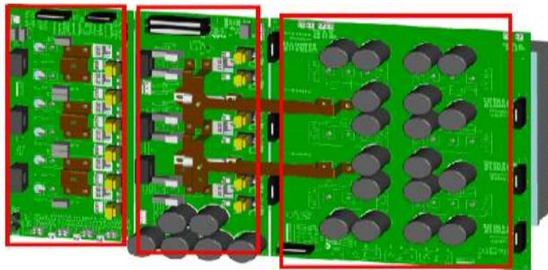
Figure 2-9: 10 ~ 40KVA rectifier, inverter and static bypass module
