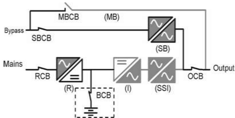
Figure 2-4: Bypass Mode
