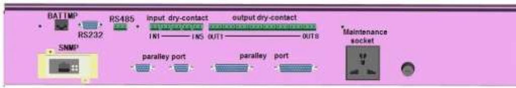
Figure 7-4: Communication Module of 60~120KVA UPS
