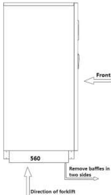
Figure 3-7: Carry of 60~120KVA (Unit: mm)
