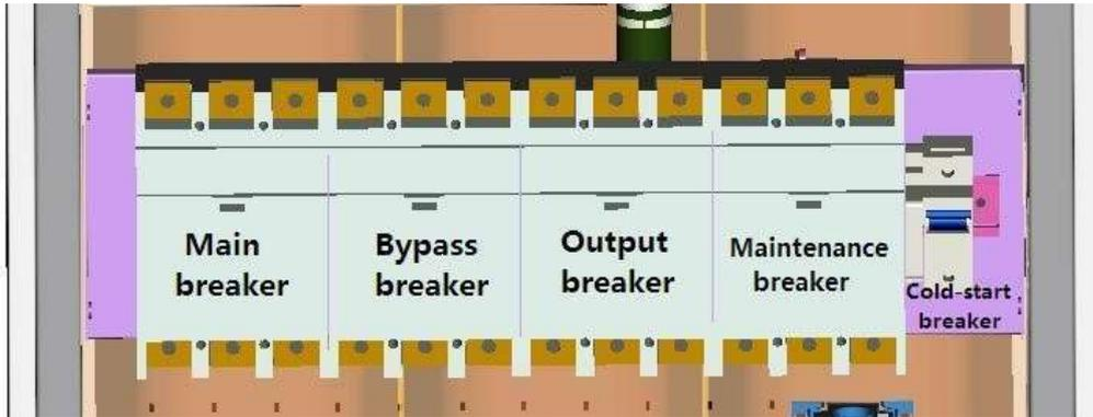
Figure 2-18: 60KVA UPS diagram of load switch
