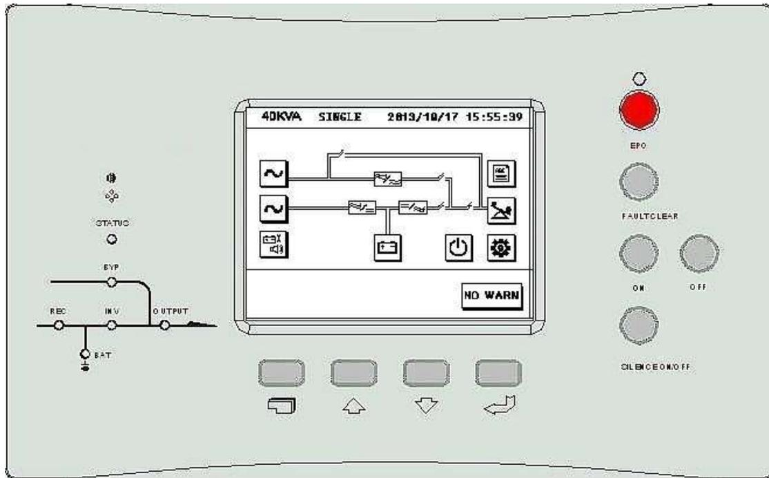
Figure 5-1: Operation Control and Display Panel of UPS
